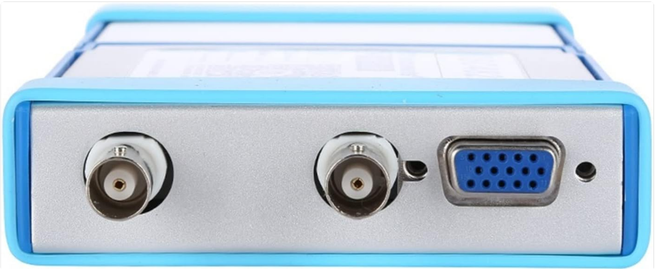
Image: The front panel of the OSC482, clearly showing the two BNC connectors for oscilloscope channels A and B, and the DB15 interface for logic analysis and signal generation.
