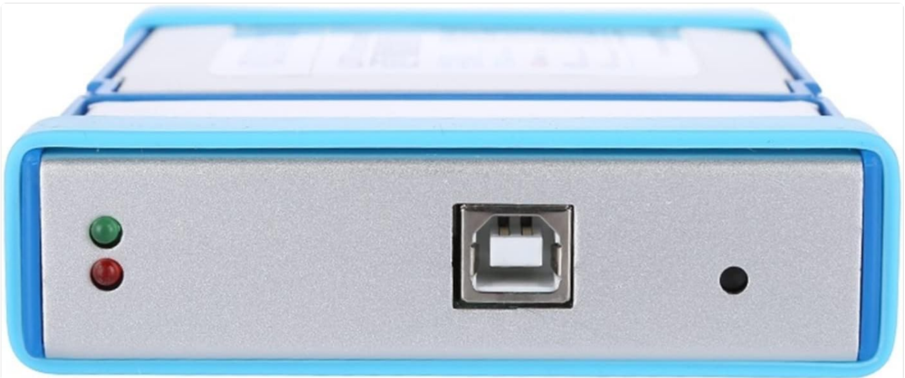
Image: The rear panel of the OSC482, displaying the USB B type port for PC connection, and the red Power LED and green Status LED.
