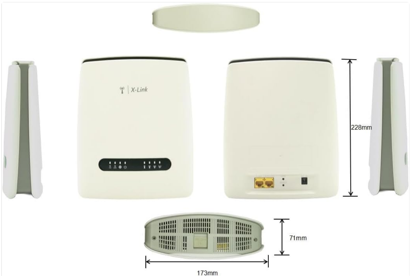
Figure 6: Top, front, side, and bottom views of the X-Link AX3000 Router, showing its dimensions (228mm height, 173mm width, 71mm depth) and port configuration.
