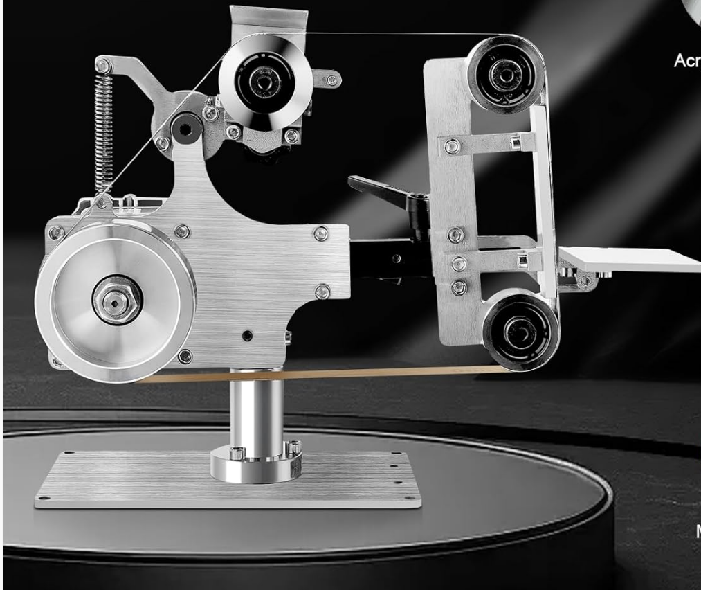
Figure 2.7: Close-up of product details, showing the Al-alloy driving wheel, the 30x0.98 inch abrasive belt, and the motor driver for convenient control.
