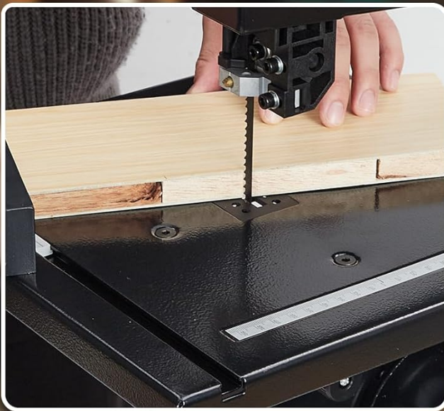
Figure 4.4: Examples of various cutting operations possible with the bandsaw, including straight line cuts, intricate curve cuts, and precise multi-angle cuts, demonstrating its versatility for woodworking projects.
