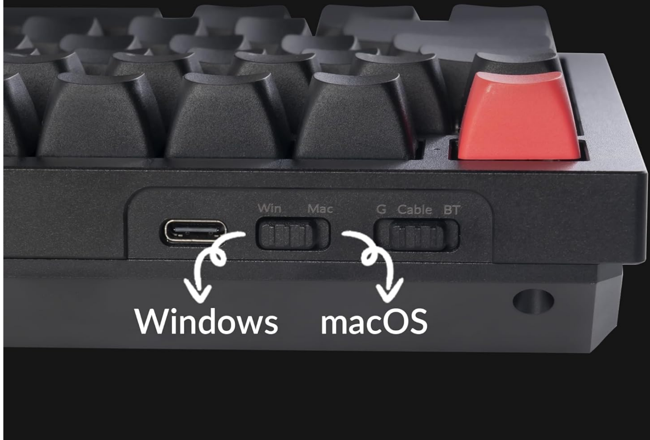
Figure 4: OS Layout Switch and USB-C Port.
