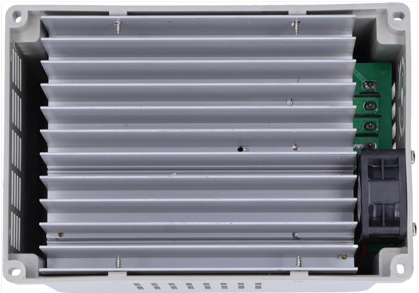
Image: Internal view of the AT5-1500X VFD, showing the heatsink fins. Keeping these clear of dust is vital for efficient cooling and preventing overheating.
