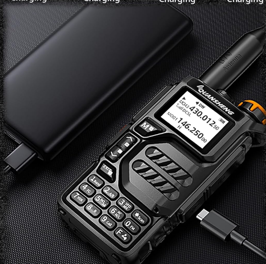
Figure 4: The UV-K5 radio supports multiple charging modes, including USB-C, PC USB, power bank, and car charging.
