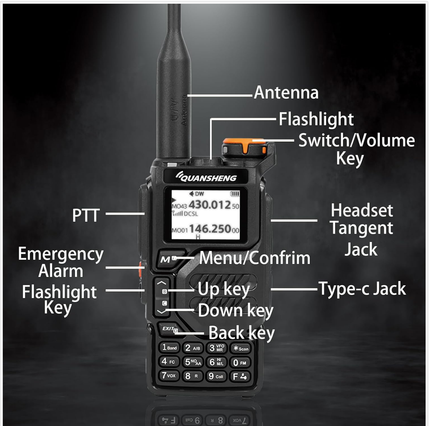
Figure 2: Quansheng UV-K5 Radio with labeled components including Antenna, Flashlight, Switch/Volume Key, PTT, Emergency Alarm/Flashlight Key, Headset Tangent Jack, Menu/Confirm, Up Key, Down Key, Back Key, and Type-C Jack.
