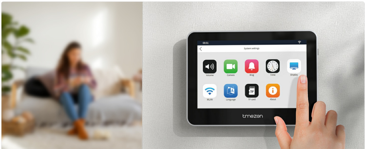
Figure 4.6: Access WLAN settings from the monitor's system menu to connect to your home WiFi network.
