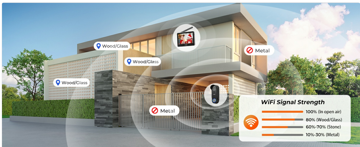
Figure 4.4: Consider material interference when placing units. Signal strength is strongest in open air, moderate through wood/glass and stone, and weakest through metal.
