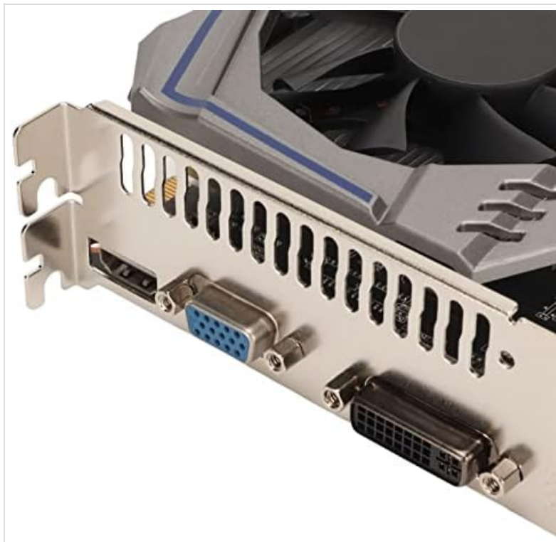
Image: A close-up view of the graphics card's output panel, showing the HDMI, VGA, and DVI ports for connecting various display types.
