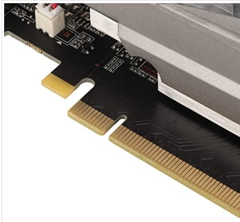
Image: A detailed view of the PCI Express connector on the graphics card, which connects to the motherboard slot.
