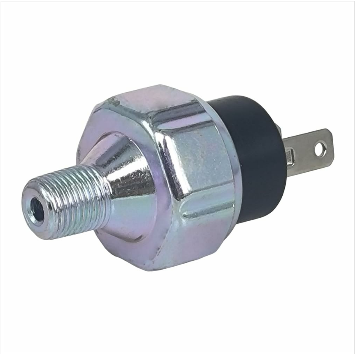
Figure 2: Side view of the sensor, highlighting the 1/8-27NPT threaded connection for installation into the engine block or oil gallery.
