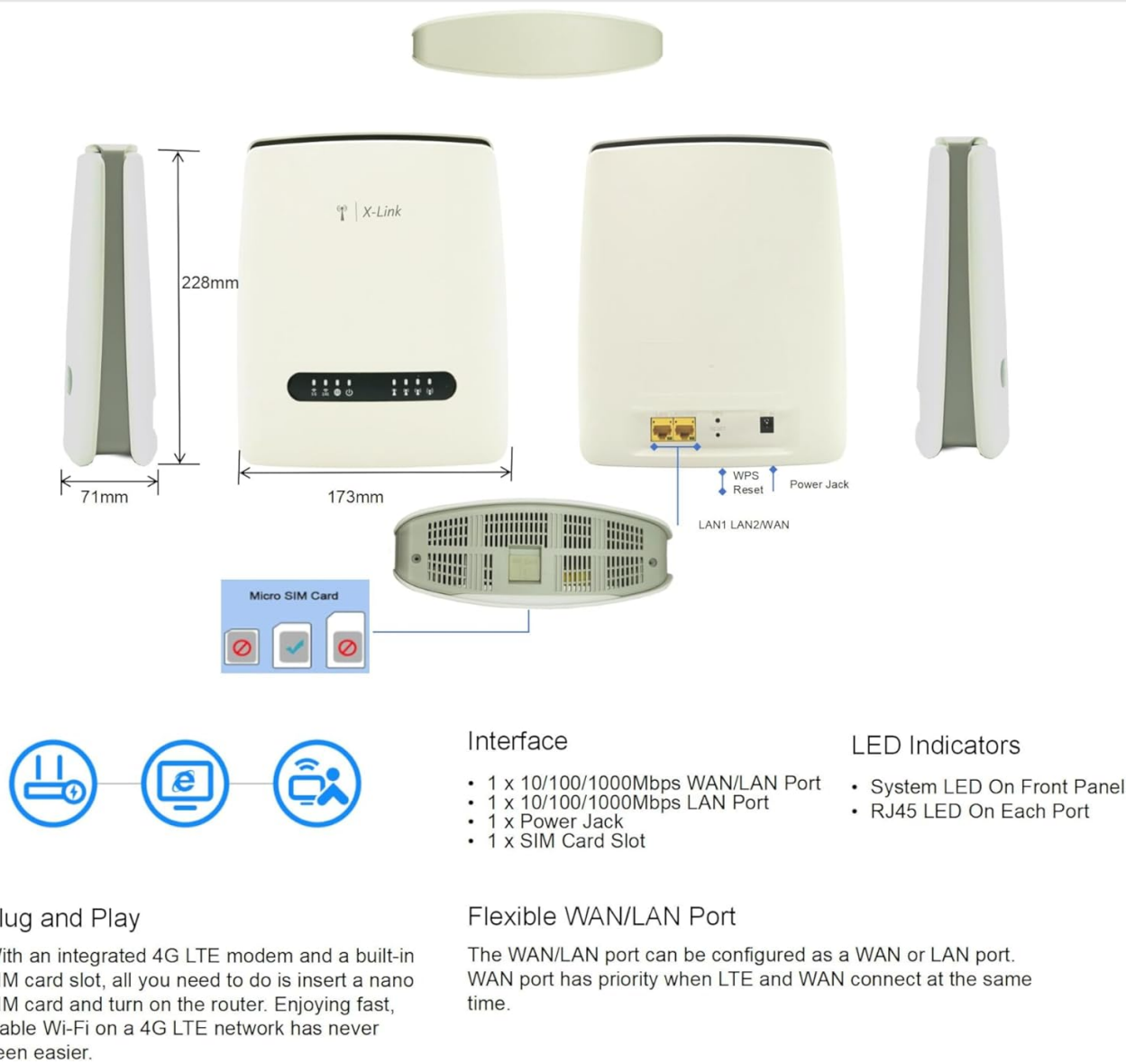
Figure 2.2.3: Router Dimensions, Interfaces, and LED Indicators. Provides a detailed diagram of the device's physical layout, including port labels and LED functions.
