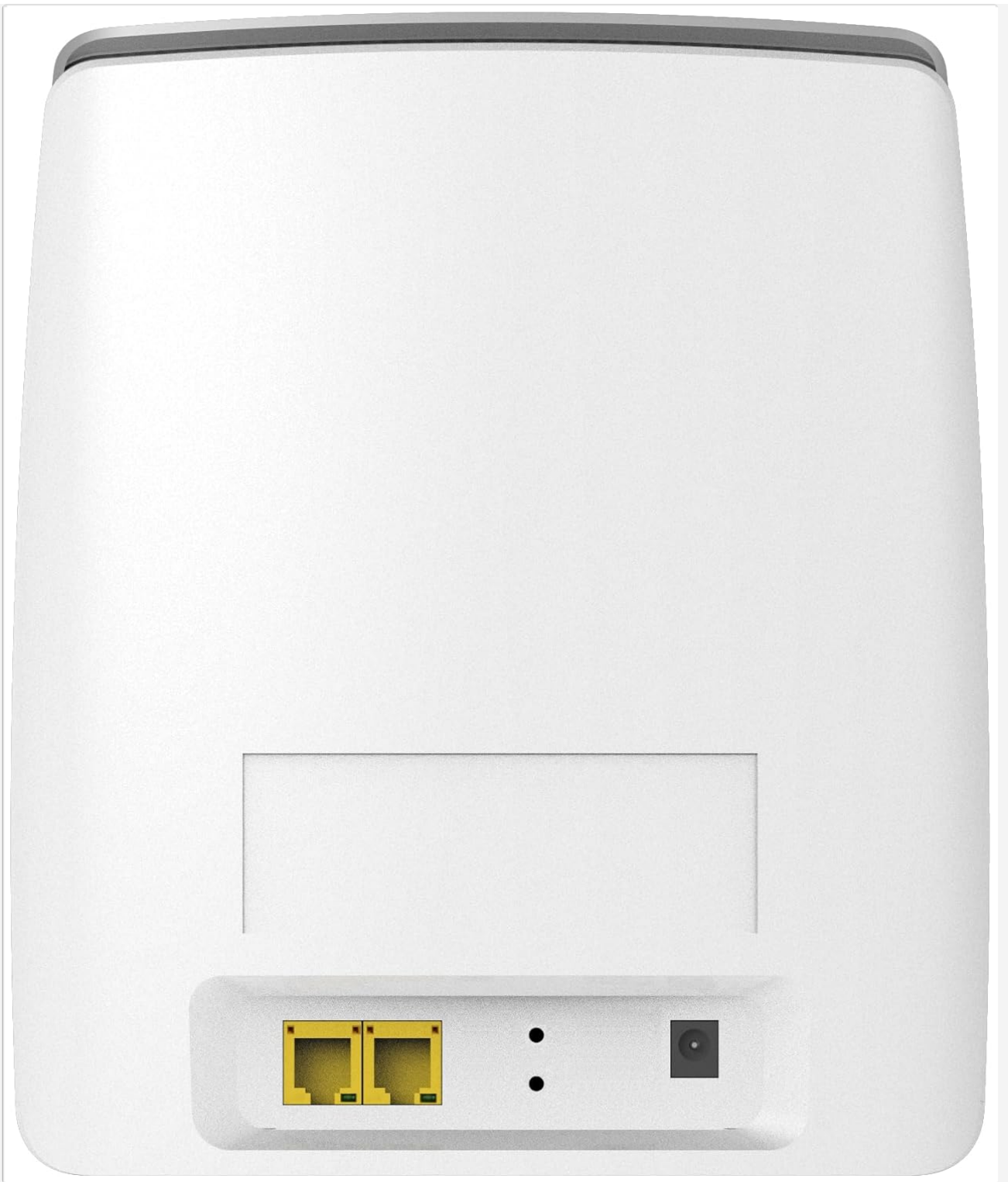
Figure 2.2.2: Back View of the Router. Displays two Gigabit Ethernet ports (LAN/WAN) and the power input jack.
