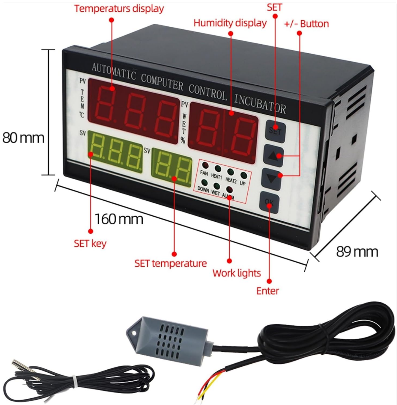
Image 2: Perspective view of the MMUNNA XM-18 controller showing its depth and the included temperature and humidity sensors. The controller measures approximately 160mm wide, 80mm high, and 89mm deep. Key interface elements like the temperature display, humidity display, SET button, +/- buttons, work lights, and enter button are also indicated.
