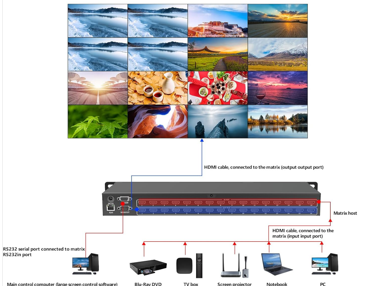
Image: A connection diagram illustrating how to connect various HDMI sources (PC, Notebook, Screen projector, TV box, Blu-ray DVD) to the input ports and how the output ports connect to a large screen display, along with RS-232 serial port connection.
