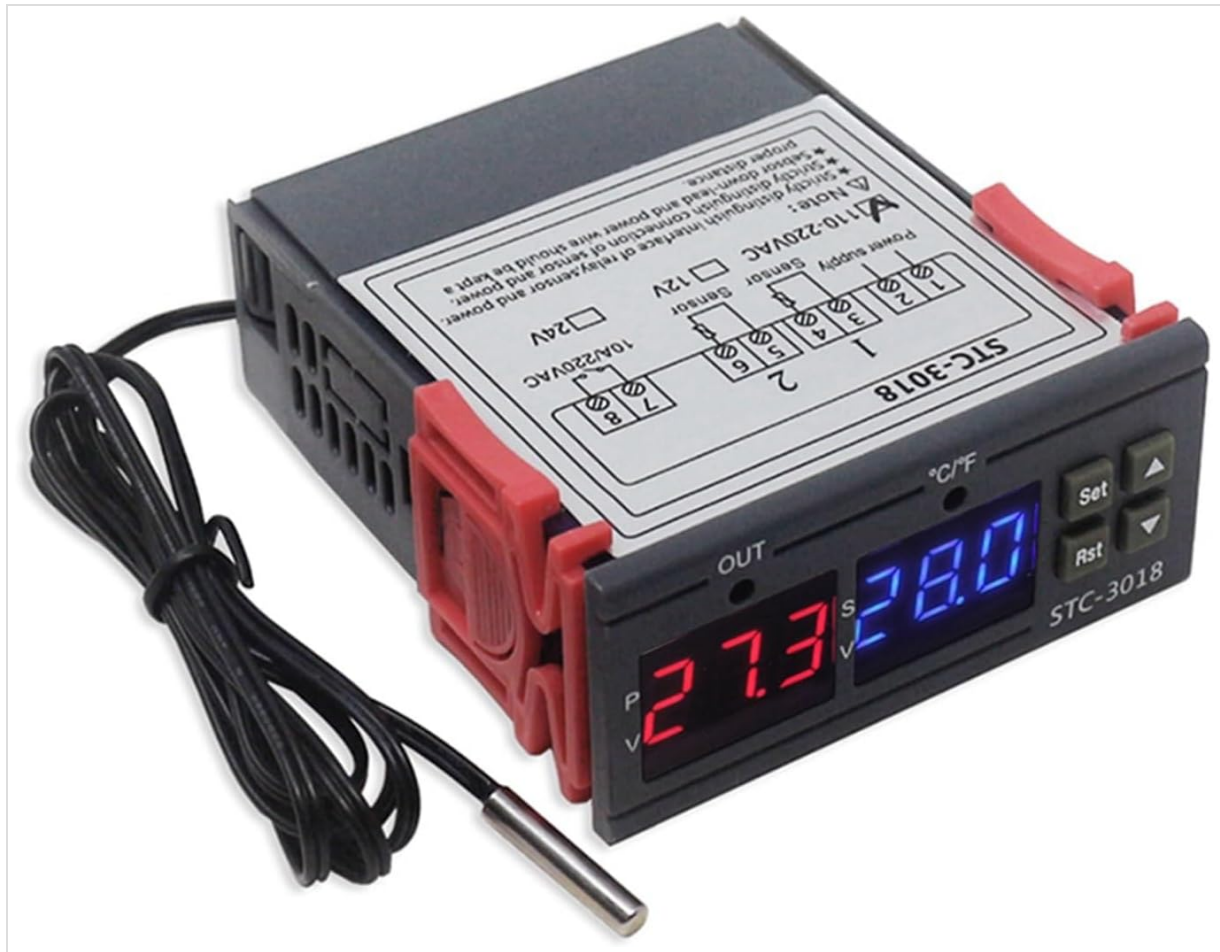
Image: Top view of the STC-3018 controller showing the display, buttons, and a label with wiring instructions and safety notes. The label indicates power supply options (110-220VAC, 12V, 24V) and relay outputs (10A/220VAC). A temperature probe is connected to the device.
