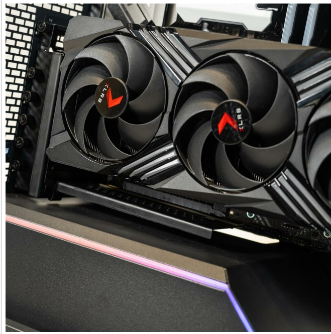
Image 4.1: Example of a graphics card vertically mounted with the bracket.
