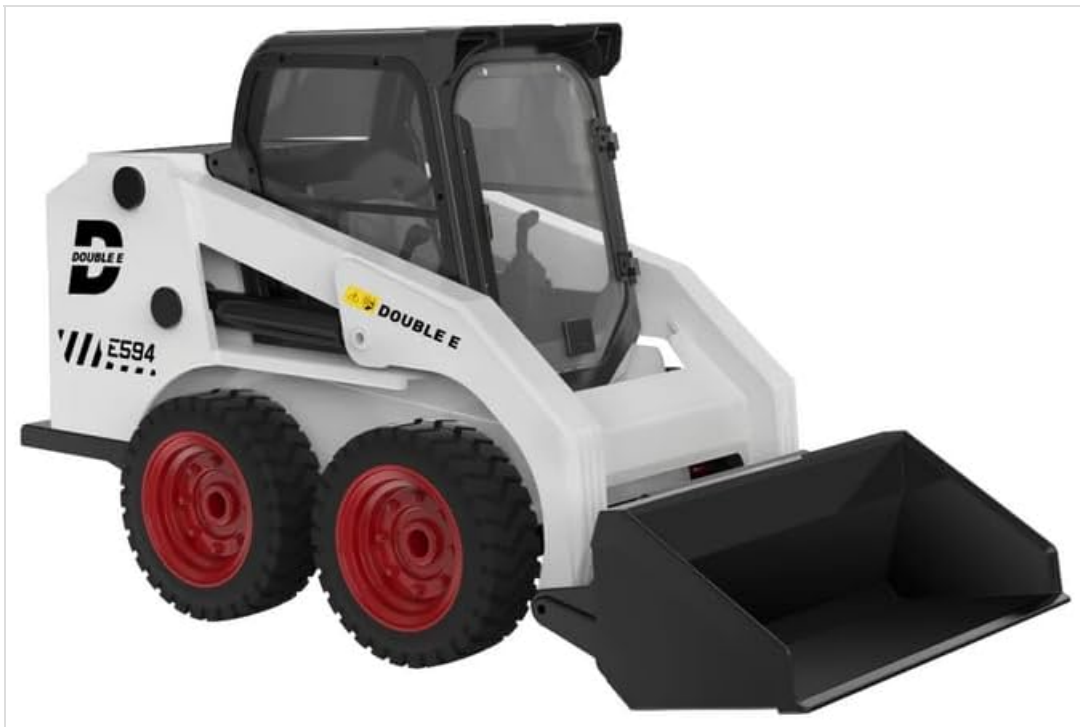
Figure 3: The s-idee® E594-003 Compact Loader with its bucket in the lowered position, ready for scooping material.
