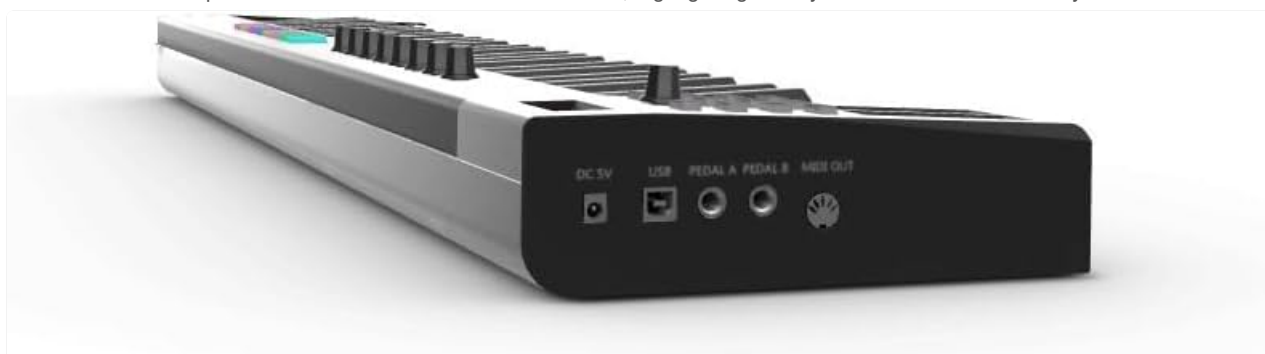
Rear view of the Worlde Blue Whale-61, showing the DC 5V power input, USB port, Pedal A and B inputs, and MIDI OUT port.
