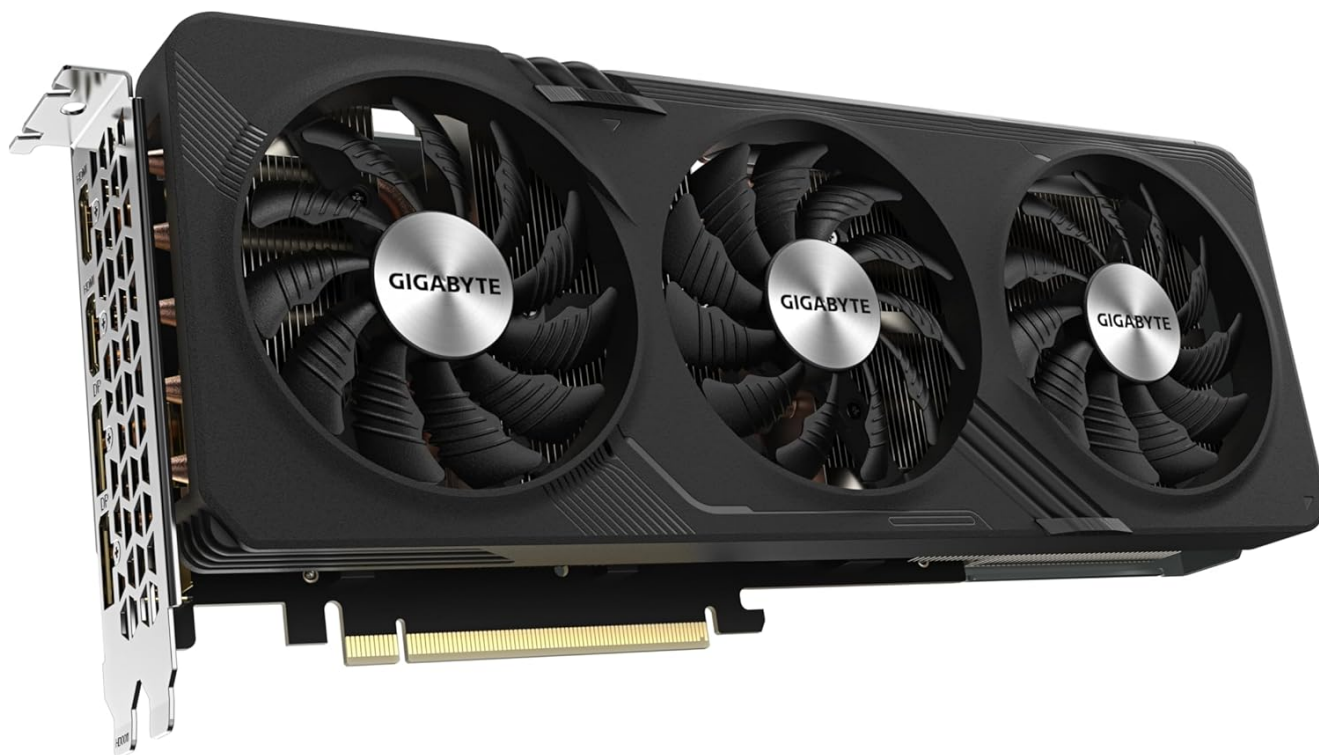
Figure 2: Front view of the graphics card, showing the triple fan design.
