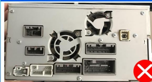
Image 3.1: Diagram showing different types of original car radio back interfaces (A, B, C). Option A, with a specific connector layout, is compatible. Options B and C are not compatible with the provided wiring harness.
