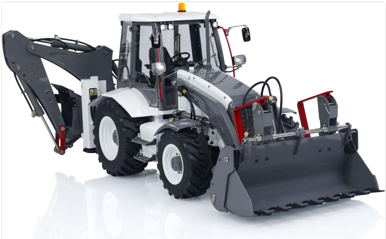
Figure 5.4: The Aoue BL71 configured for backhoe operation.
