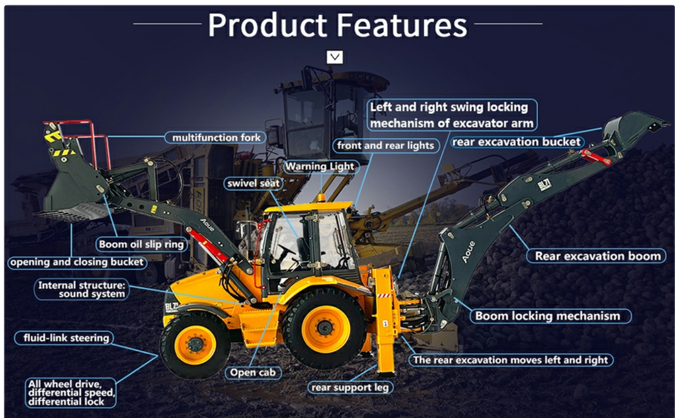
Figure 3.1: Key features and components of the Aoue BL71 Backhoe Loader.
