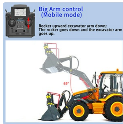
Figure 5.2: Remote control input for raising/lowering the front loader arm.
