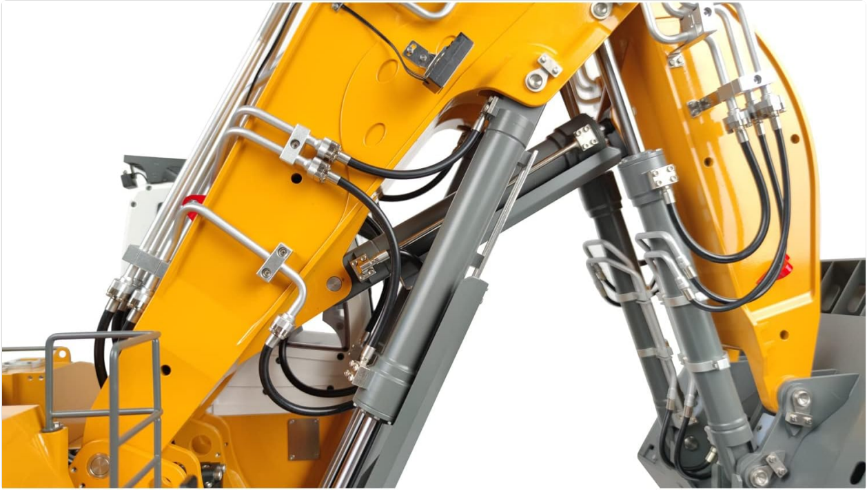
Image: Detailed view of the excavator's hydraulic cylinders and associated plumbing, critical for its operation.
