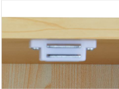
Figure 4.3: Detail of the magnetic latch mechanism that keeps the doors closed.
