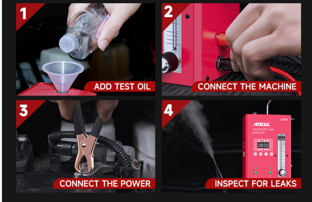
Image 5.1: A simplified visual guide showing the four steps for quick setup: 1) Fill test oil (baby oil recommended), 2) Disconnect the pipe to be tested, 3) Connect the detector to a DC 12V battery and choose work mode, and 4) Inspect for smoke to identify leak points.
