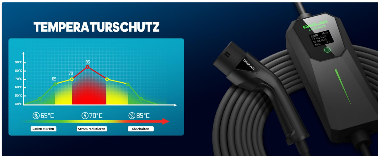
Figure 5.2: Graph illustrating the temperature protection mechanism: charging starts below 65°C, current is reduced between 70°C and 85°C, and the unit shuts down above 85°C.
