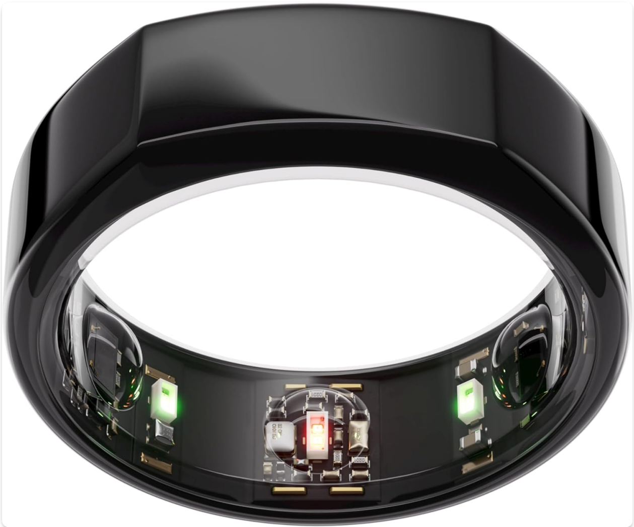
Figure 1: The OURA Ring Gen3 Heritage, highlighting its internal sensors.
