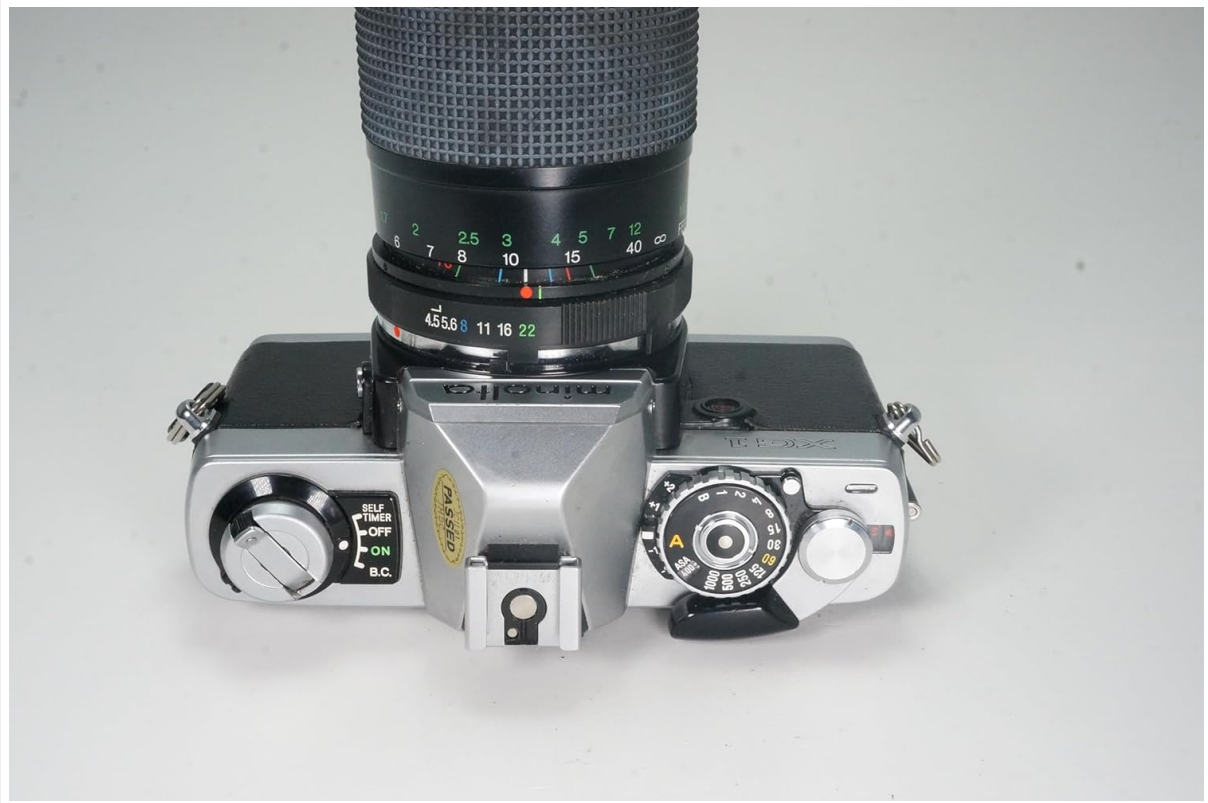
Figure 3: Top view of the Minolta XG-1, illustrating the shutter speed dial (right), film advance lever (right), and the hot shoe for flash (center).
