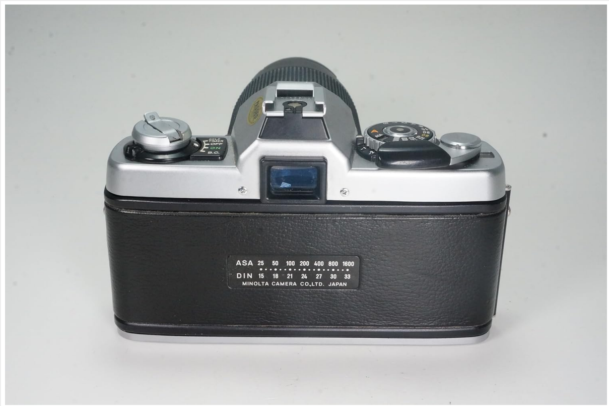
Figure 2: The back of the Minolta XG-1 camera, displaying the ASA and DIN film speed settings. Adjust the dial to match your film's sensitivity.
