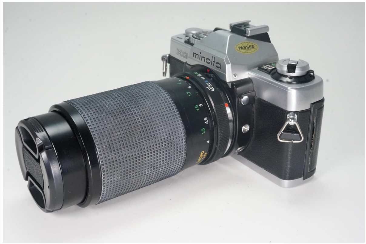
Figure 4: Side view of the Minolta XG-1 camera and its zoom lens. The focus and zoom rings on the lens are visible for manual adjustment.
