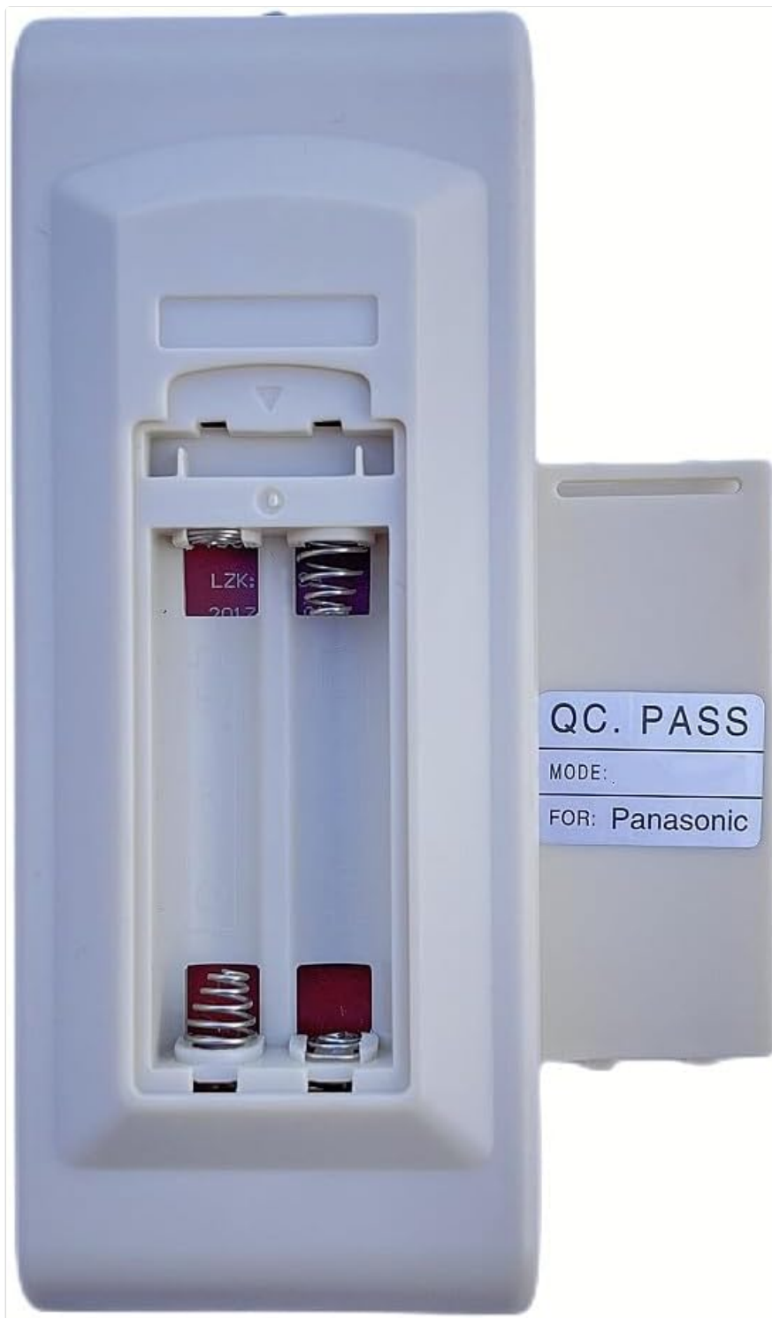
Image: Back of the remote control with the battery compartment open, illustrating where to insert batteries.
