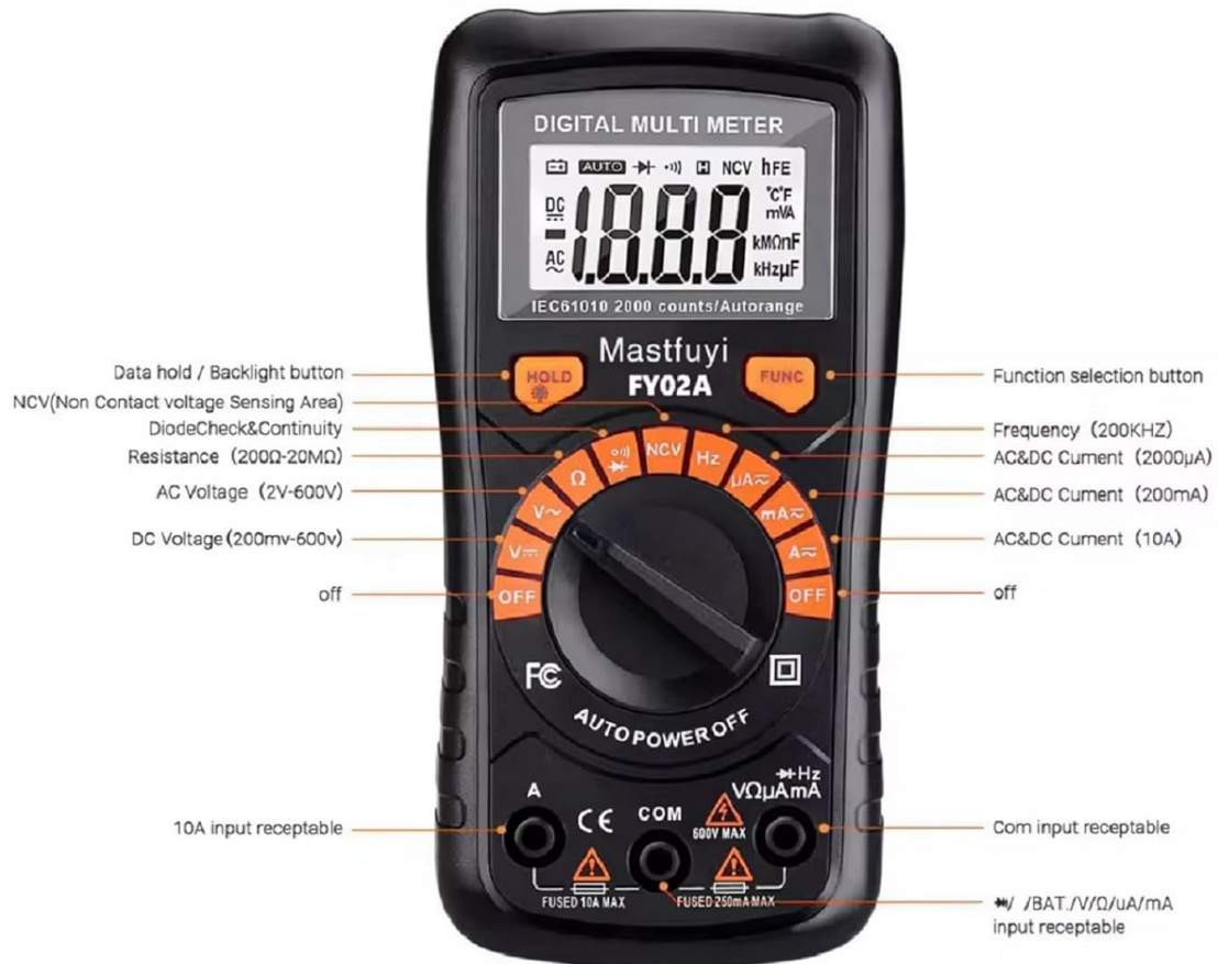
Image: Detailed diagram of the Mastfuyi FY02A multimeter, highlighting the LCD display, function dial, input jacks, and control buttons.
