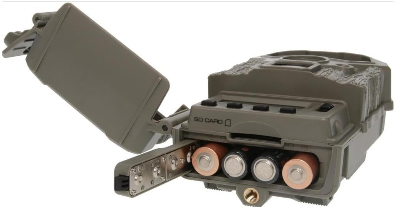
Image: Internal view of the camera, illustrating the battery and SD card insertion points.
