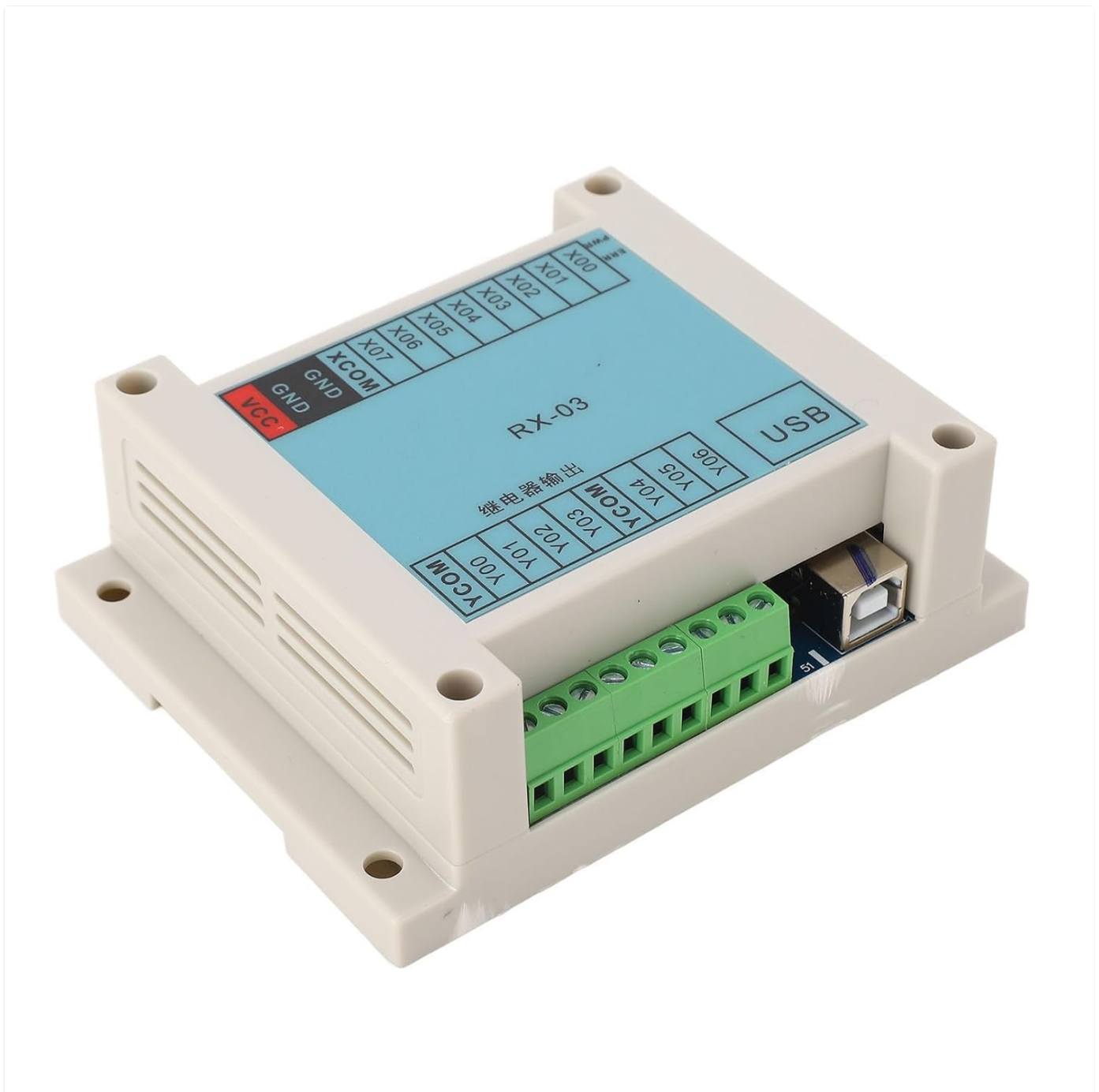
Figure 1: Agatige RX-03 PLC Control Board, front view showing input/output terminals and USB port.
