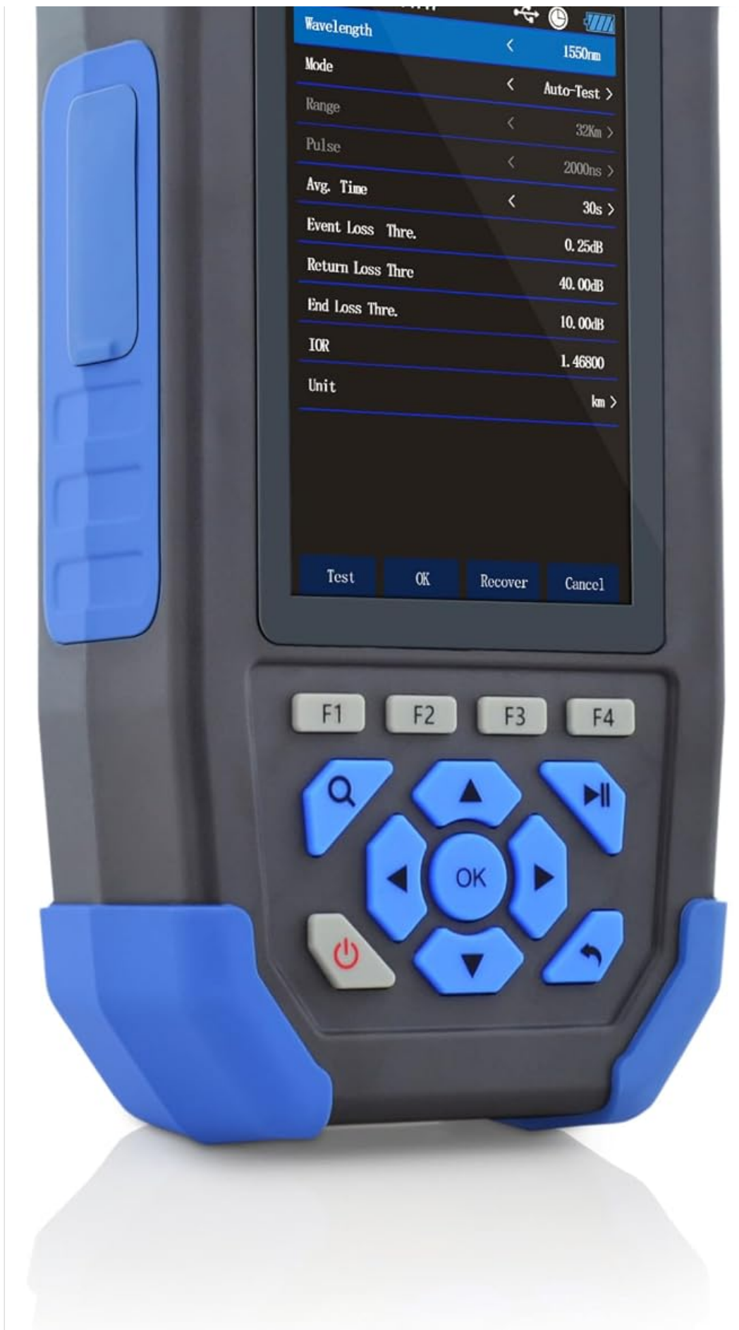
Image: The OTDR settings screen, displaying options for Wavelength, Range, Pulse, Average Time, Event Loss Threshold, Return Loss Threshold, and Unit settings.
