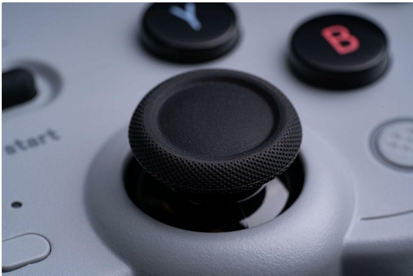
Figure 7: A close-up view of the Hall Effect Joystick on the 8Bitdo Pro 2 Controller, highlighting its advanced magnetic sensing technology.
