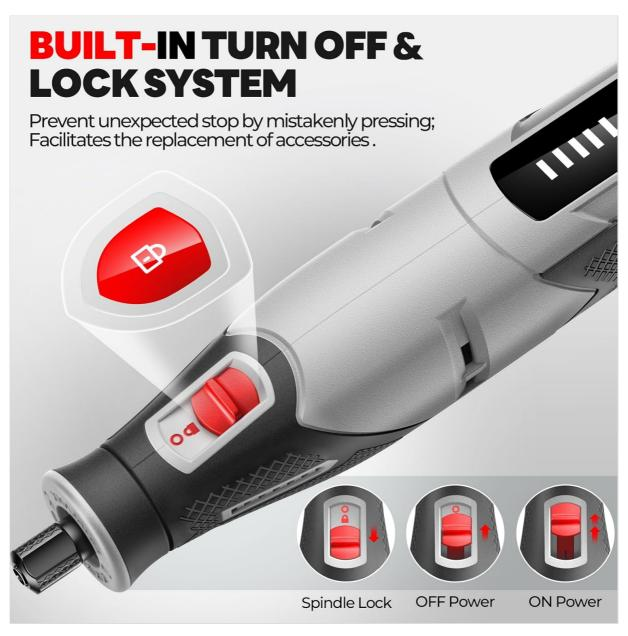
To attach or change an accessory, ensure the tool is powered off and the spindle is locked. Push the power on/off and spindle lock slider to the 'Lock' position (rear position). This will prevent the shaft from rotating. Loosen the
