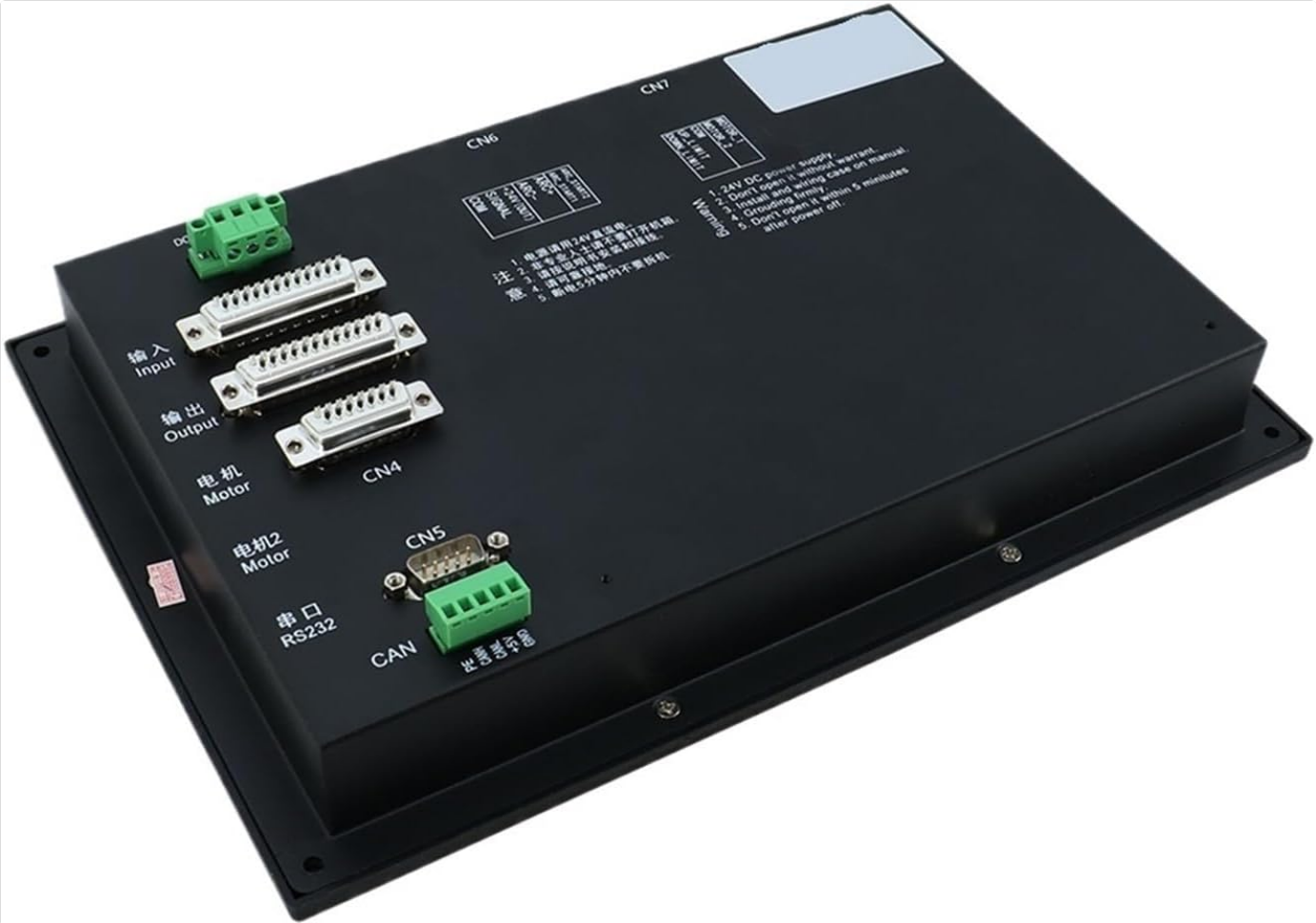
Figure 2.3: Included connectors for the F2100B system, comprising D-sub 25-pin and 15-pin connectors, along with green terminal blocks for secure wiring.
