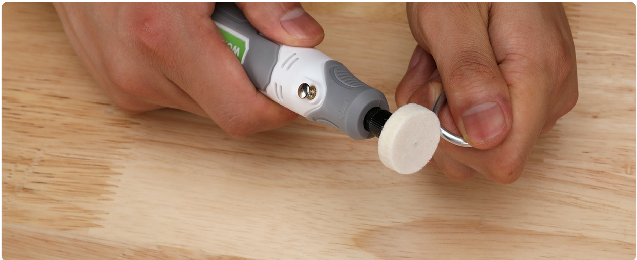
Image: A three-step visual guide demonstrating how to change accessories on the rotary tool: 1. Press the shaft lock, 2. Unscrew the collet nut, 3. Tighten the black nut after inserting the new accessory.
