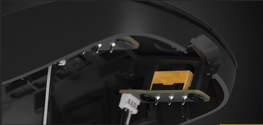
Figure 3.3: The swappable main button switch design, allowing for personalized click feel by replacing switches.
