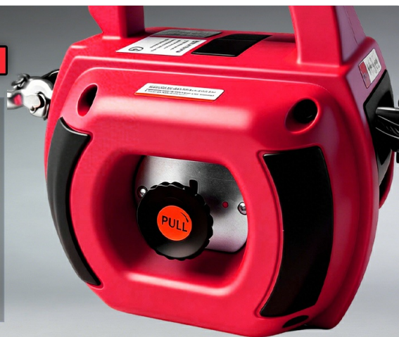
Image 3.3: Illustration of the free-spool clutch knob. Pulling the knob and turning clockwise allows free rotation, while turning counter-clockwise locks the drive rod.
