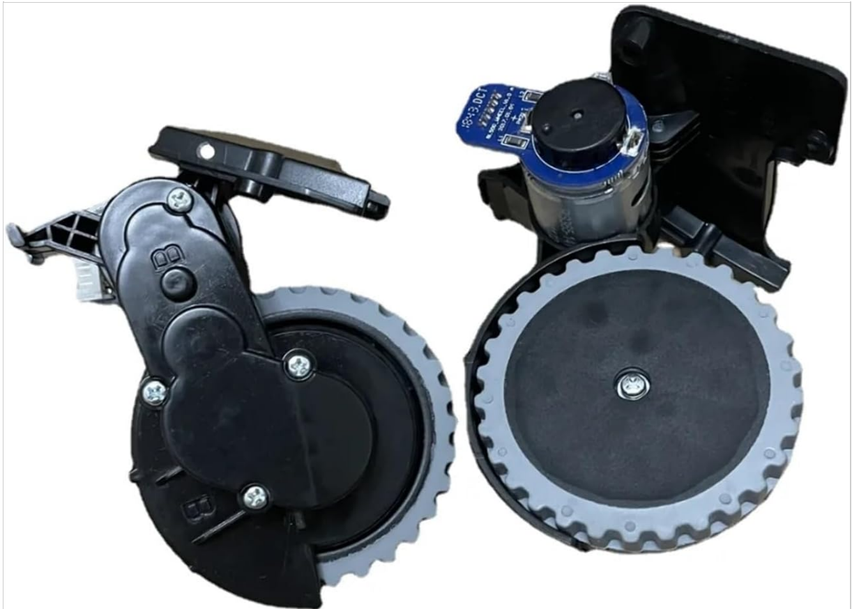
Image: Two replacement wheel motors, showing their design and components. One is marked 'L' for left and the other 'R' for right, indicating their intended installation side.
