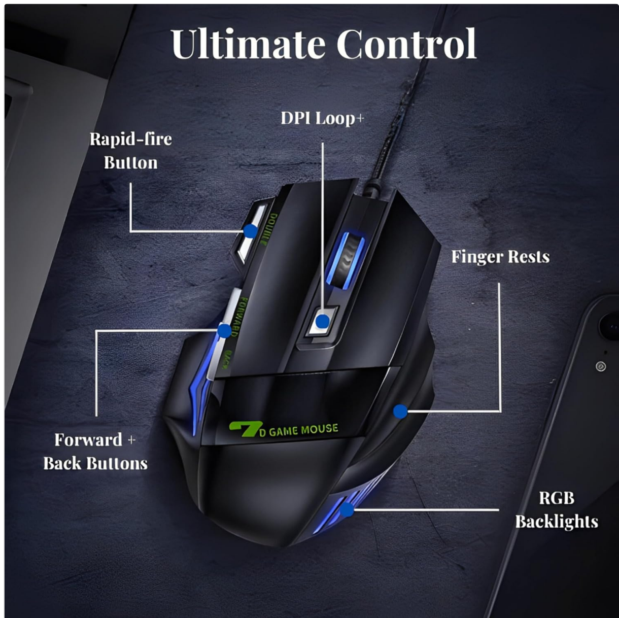
Image: Overview of the Nexurion Reaper Z Pro Gaming Mouse, highlighting its key features including the Rapid-fire Button, DPI Loop+ button, Finger Rests, Forward + Back Buttons, and RGB Backlights.
