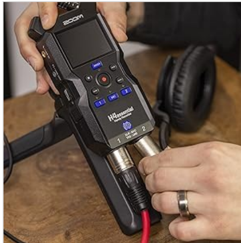
Figure 7: A user connecting XLR cables to the combo inputs of the H4essential, demonstrating external microphone connectivity.
