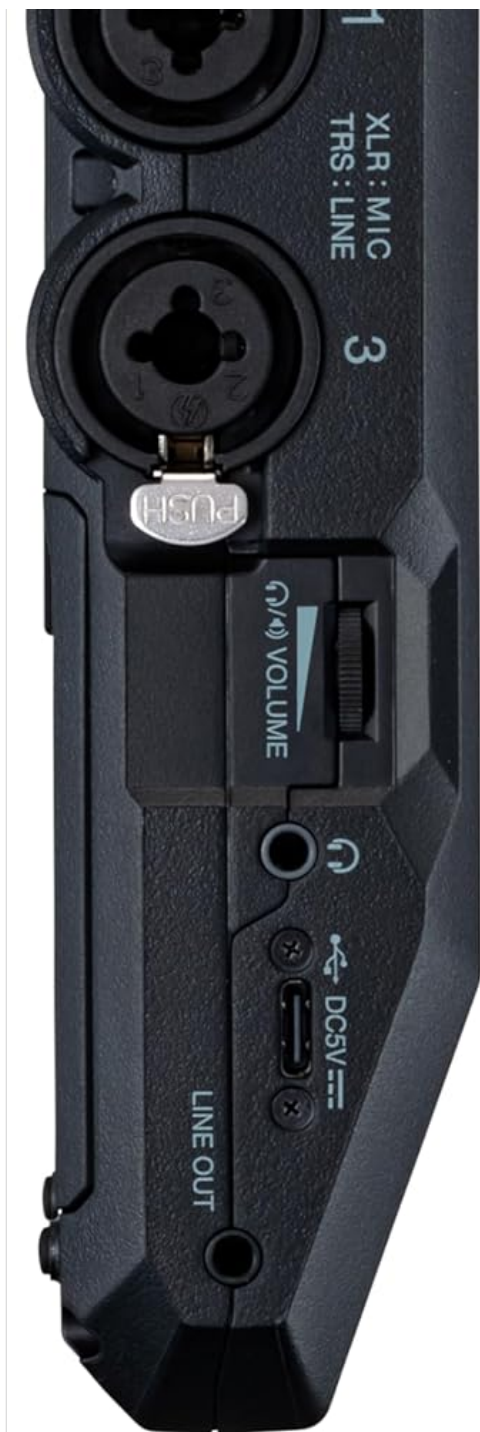
Figure 3.2: Left side of the H6essential, featuring XLR/TRS combo inputs 1 and 3, a volume slider, headphone jack, DC 5V power input, and line out port. These ports are used for connecting external microphones and monitoring audio.
