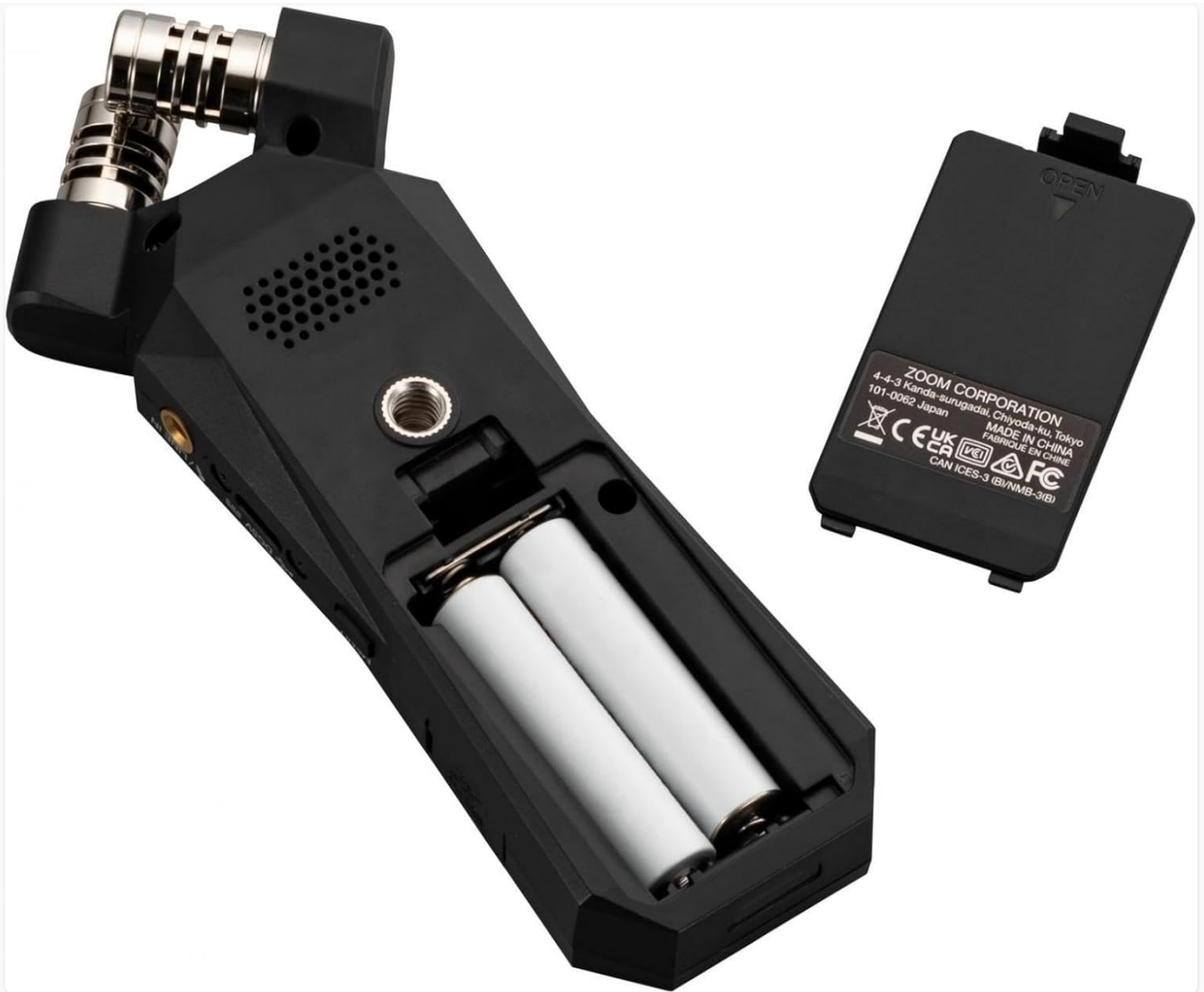
Figure 1: Rear view of the H1essential with the battery compartment open, revealing the two AAA batteries.
