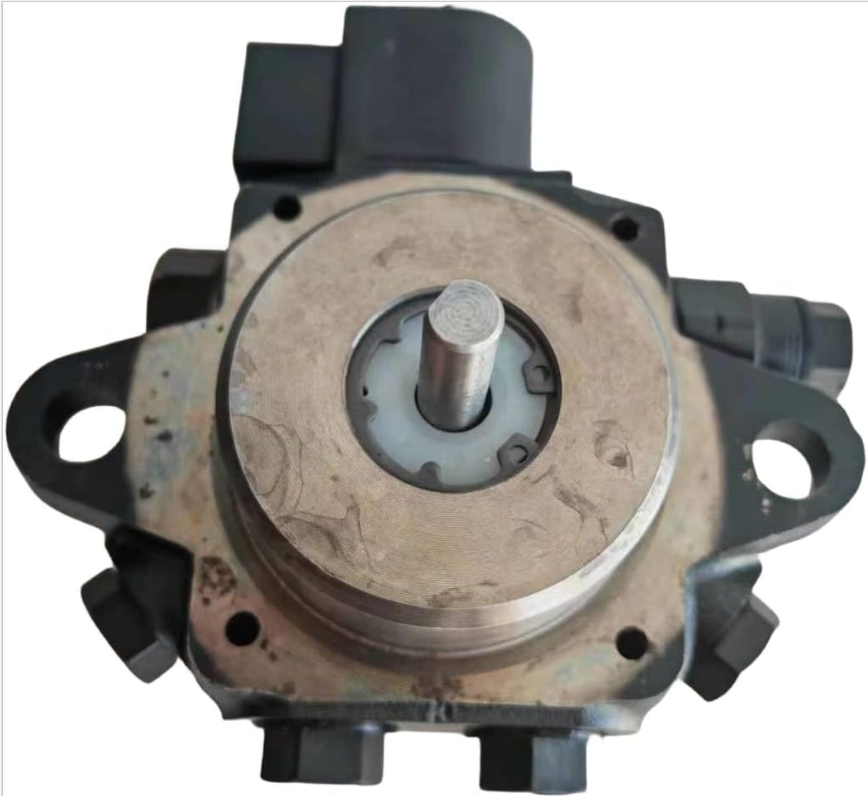
Figure 4.1: Bottom view of the SUNTEC AS47A 7432-4 oil pump. This image shows the central drive shaft and the surrounding mounting points, which are essential for proper alignment and secure attachment to the burner motor.
