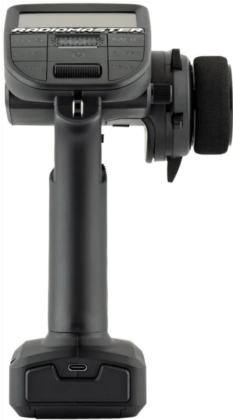
Figure 3.5: Front view of the RadioMaster MT12, showing the grip and the USB-C port located at the base for charging and data transfer.
