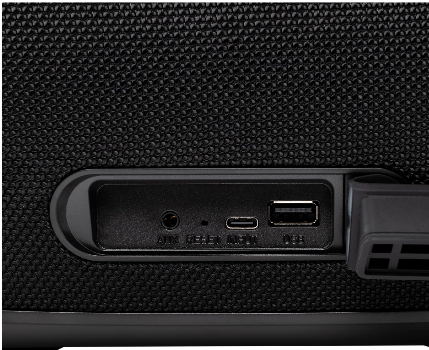
Figure 4.3: Close-up of the protected input/output ports on the rear of the speaker.
