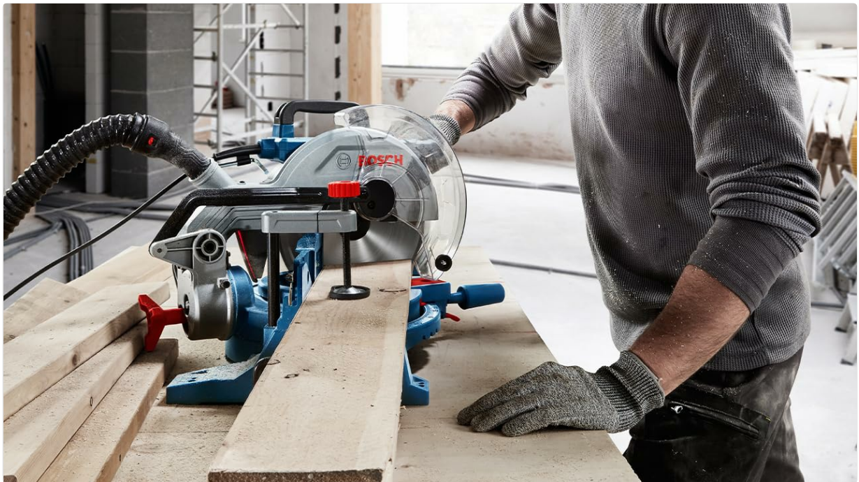
Image 5.1: An operator demonstrating the use of the mitre saw for cutting a wooden beam.
