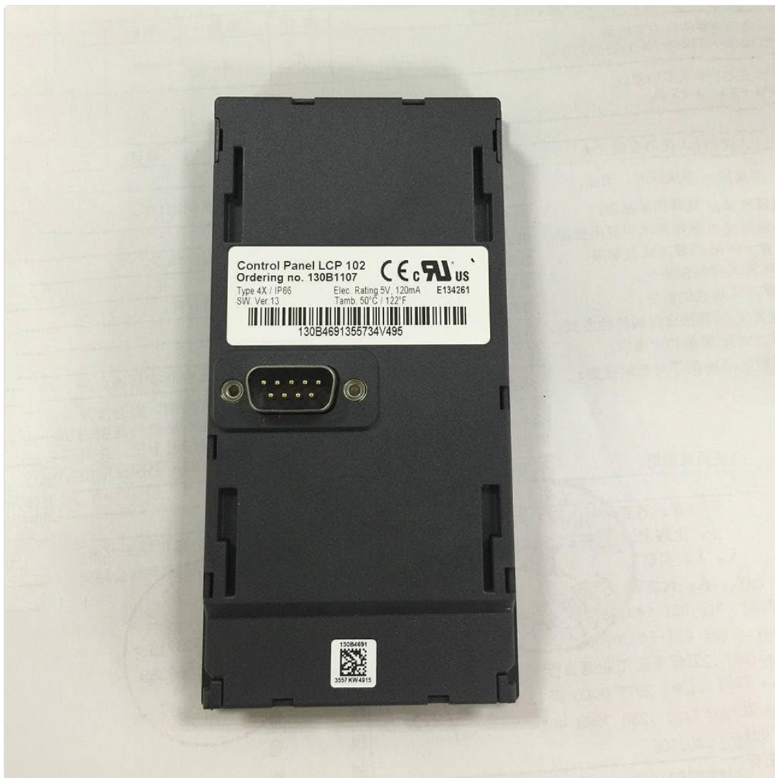
Figure 2: Rear view of the LCP102 LCD Operation Panel. This image shows the multi-pin connector for inverter communication and the product label. The label indicates "Control Panel LCP 102", "Ordering no. 130B1107", "Type 4K / IP66", "Elec. Rating 5V 120mA", "Temp. 50°C / 122°F", and "SW. Ver 1.3". A barcode with the number 130B4691355734V495 and another with 13066469135573486495 are also visible.
