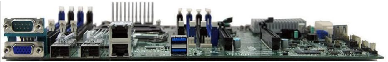
Figure 2: Rear I/O panel of the Generic MS-S1561 Server Motherboard, showing various ports including USB, LAN, and VGA.
