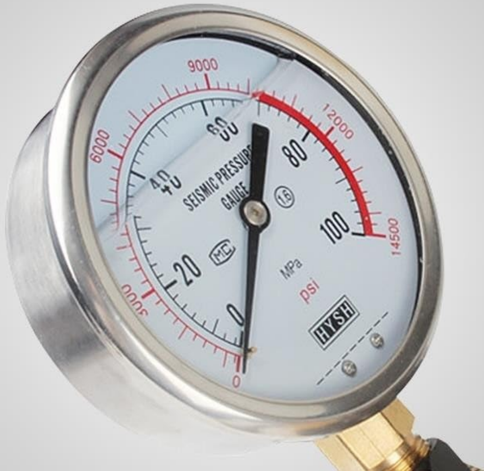
Figure 3.4: Detailed view of the shockproof pressure gauge, which provides real-time observation of pressure changes and is designed for non-explosive pump operation.
