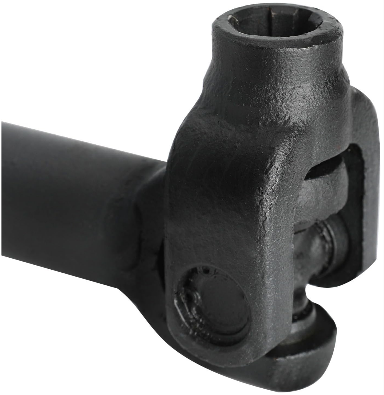
Figure 4: Close-up view of the universal joint (yoke) end of the drive shaft.
